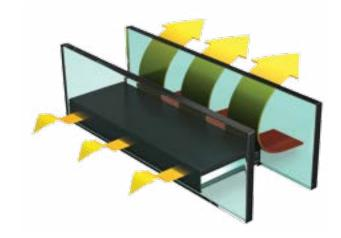
The Duralite® spacer is a component laminate design that optimizes the use of a number of spacer components. All spacers need adhesives, sealants, structural elements and
